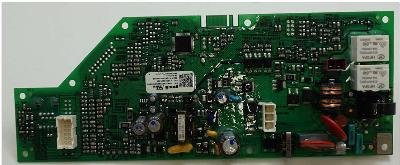
Figure 1: Front view of the WD21X24901 control board, showing various electronic components and connectors.
