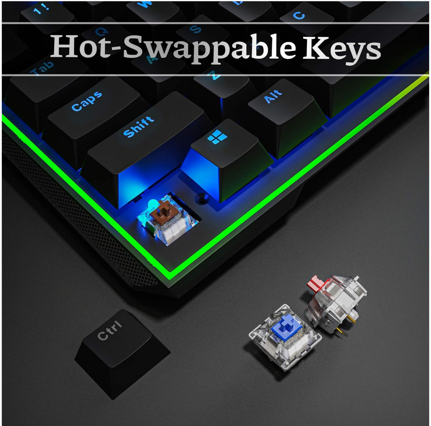
Figure 6.1: Illustration of removing a hot-swappable key switch.
