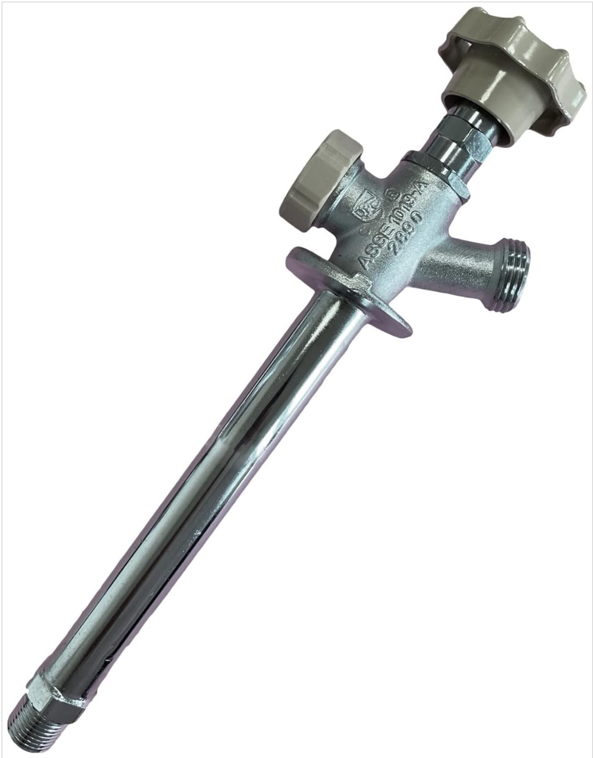
Figure 1: PROFLO PF73ASDP Anti-Siphon Sillcock. This image displays the complete sillcock unit, showing the bronze body, the multi-turn handwheel at the top, the anti-siphon cap, the 1/2-inch inlet pipe extending downwards, and the threaded hose connection at the side.
