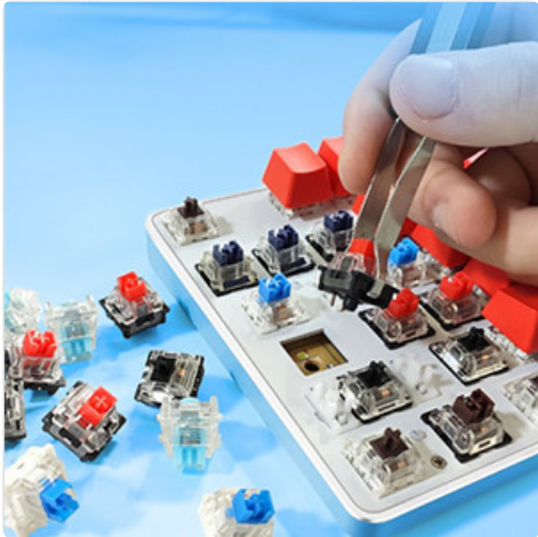
Image: A close-up showing a tool being used to remove a mechanical switch from the keyboard, illustrating the hot-swappable design.
