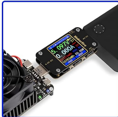
Figure 4.2: Demonstration of the voltage and current accuracy of the MakerHawk N20 compared to a professional instrument.
