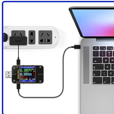
Figure 4.2: Demonstration of the voltage and current accuracy of the MakerHawk N20 compared to a professional instrument.
