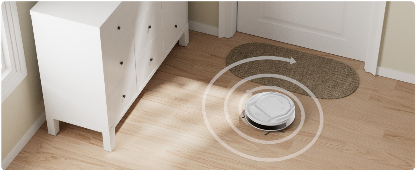
Figure 5.1: The robot automatically returns to its charging base when battery is low.
