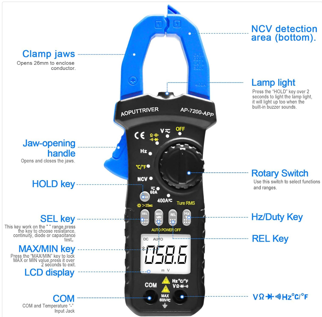
Figure 2: Front view of the clamp meter with key components labeled.
