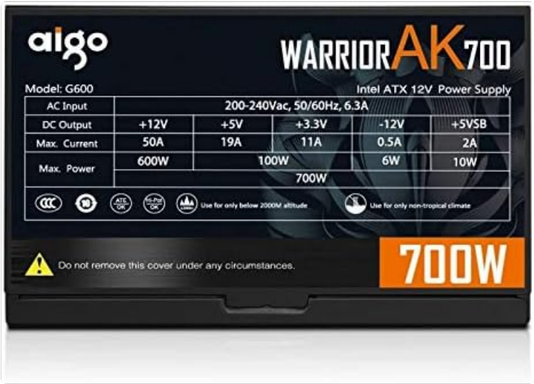
Figure 9.1: The specifications label found on the Aigo Warrior AK700 Max Power Supply.
