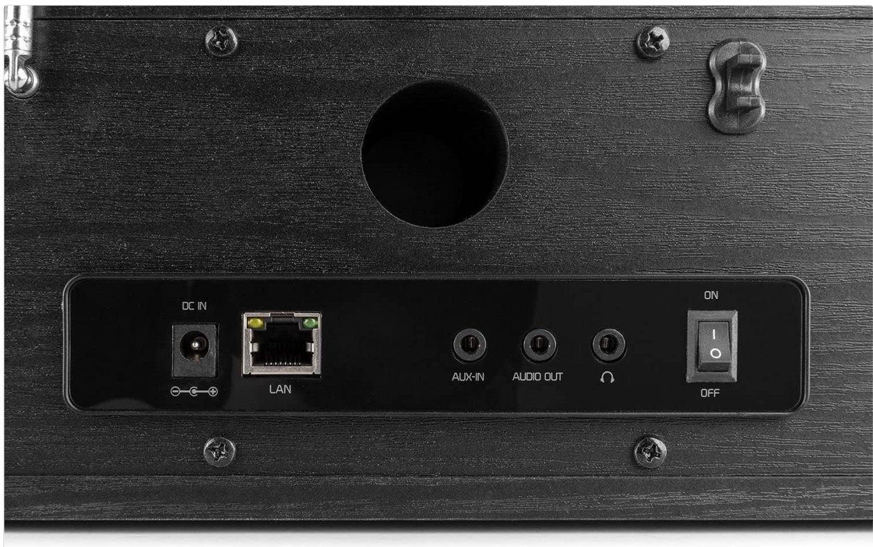
Figure 4.3: Rear panel of the Audizio Rome radio, showing DC input, LAN port, AUX-IN, AUDIO OUT, headphone jack, and power switch. These ports allow for various wired connections.
