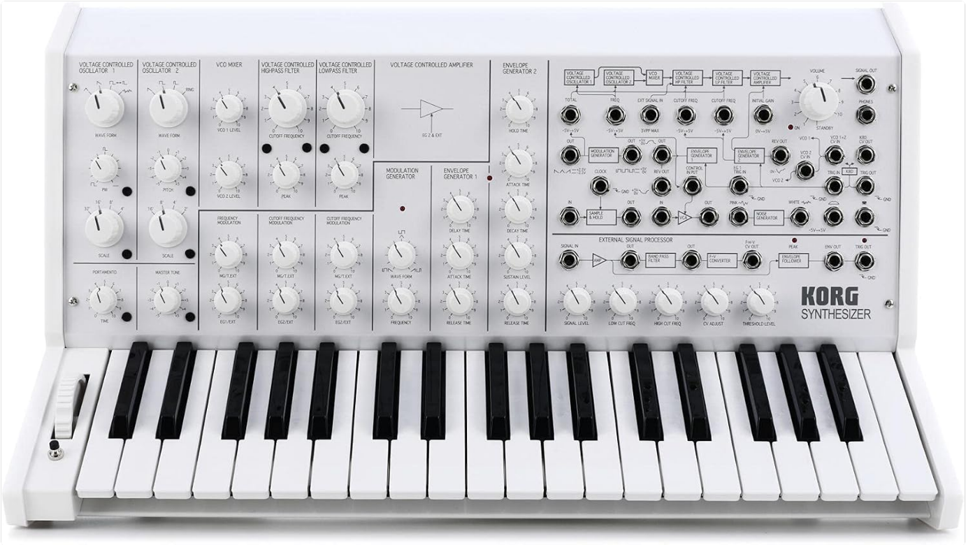
Image 1: Front panel of the Korg MS-20 FS Analog Synthesizer, showcasing the 37-key keyboard, control knobs, switches, and the patchbay section. The white finish and classic design elements are clearly visible.
