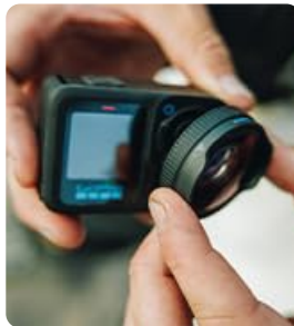
Image: Detailed view of the twisting motion required to secure the Max Lens Mod.
