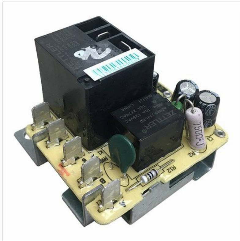
Image 2: An angled view of the time delay relay's circuit board, showing various components and connection terminals. Proper identification of these terminals is crucial for correct installation.
