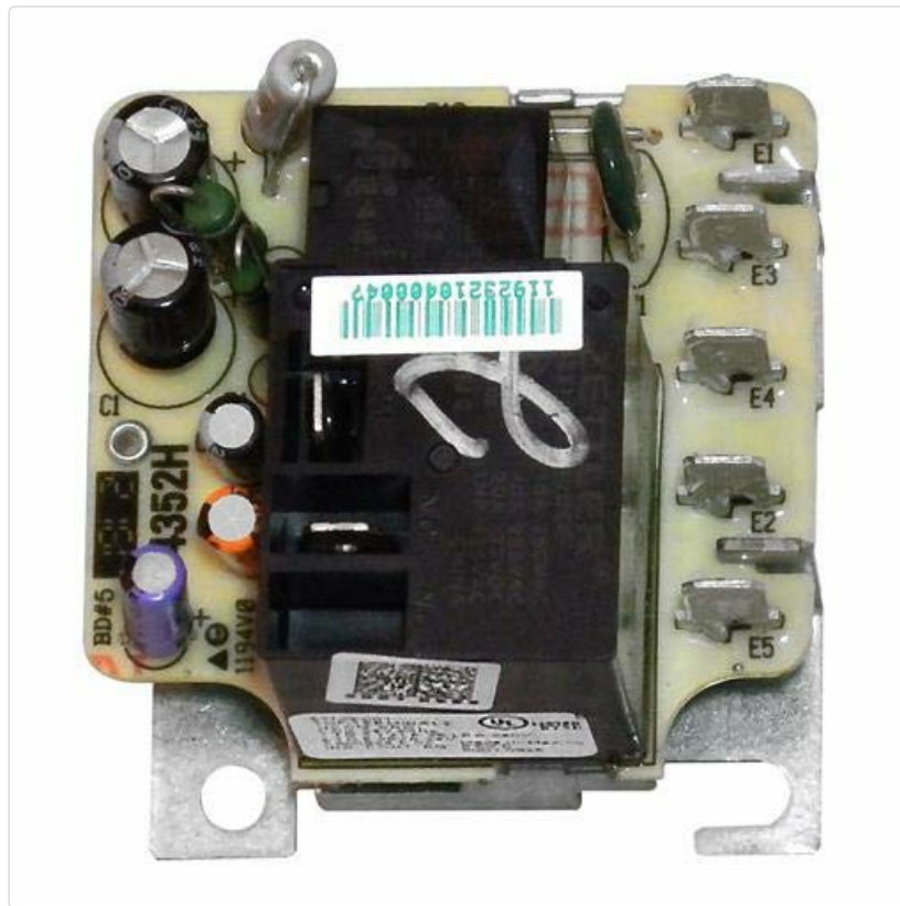
Image 4: A top-down perspective of the time delay relay's circuit board, showing the layout of the relay, capacitors, resistors, and terminal connections. This view can assist in identifying components and wiring points.
