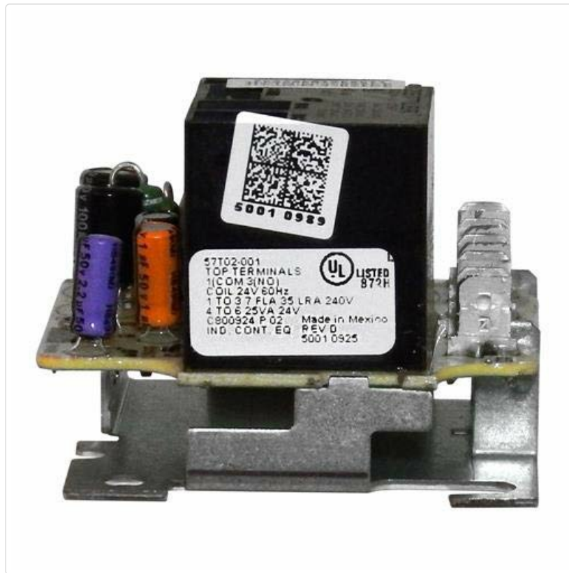
Image 3: A side view of the time delay relay, highlighting the product label with specifications such as UL listing, voltage, and current ratings. This label is important for verifying the correct part.
