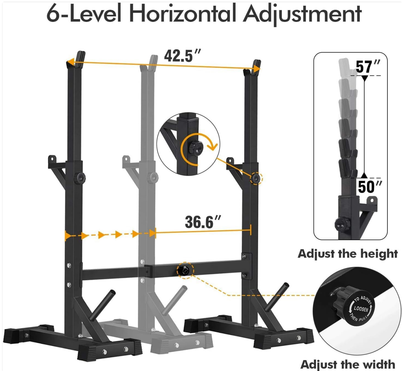
Figure 4: Adjustment Mechanisms. This image demonstrates how to adjust both the horizontal width and the vertical height of the squat rack for optimal exercise positioning.
