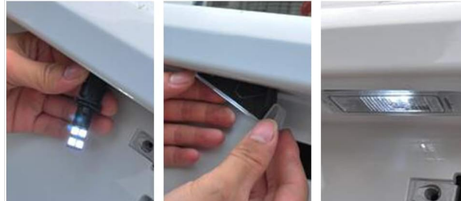
Image 6.1: Visual guide for removing the original license plate light and installing the WinPower LED replacement.
