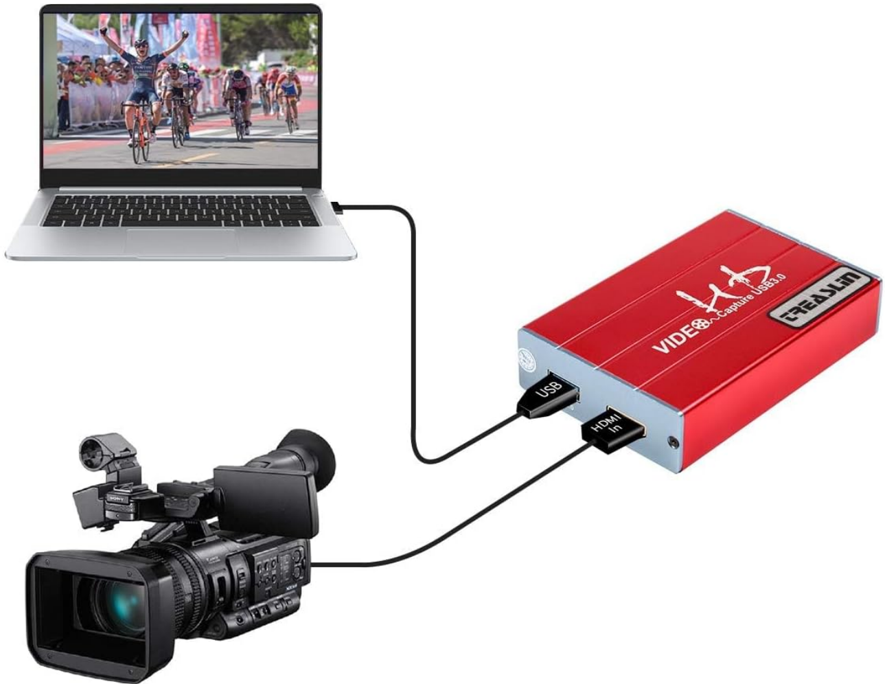
Image 4.4: Example setup for an outdoor camera live broadcast, showing a camcorder connected to a laptop via the capture card, supporting 1080P 60FPS HDMI source input.
