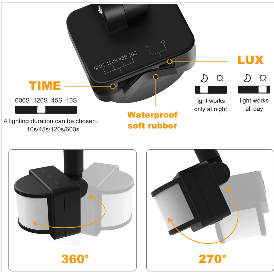
Figure 5: Detailed view of the TIME and LUX adjustment dials on the motion sensor.
