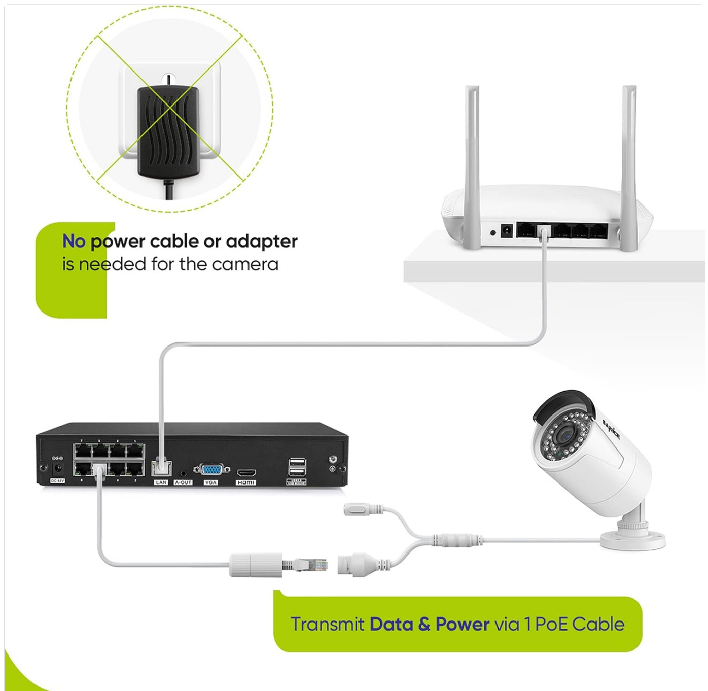
Figure 3.1: Simplified wiring with Power over Ethernet (PoE), where a single Ethernet cable transmits both data and power to the camera from the NVR.
