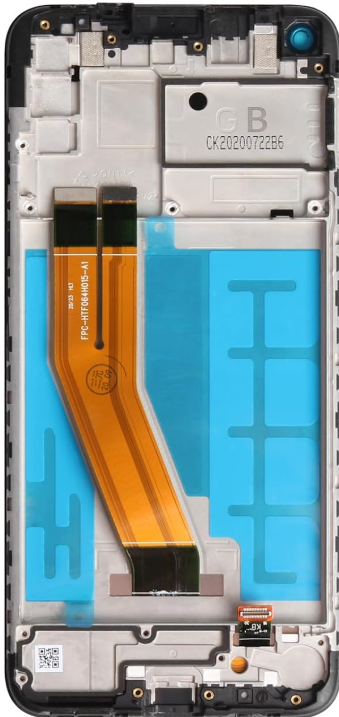
Image 4.1: Detailed view of the screen's internal components, highlighting the flex cable, connector, camera ring, and ARC frame for proper installation.
