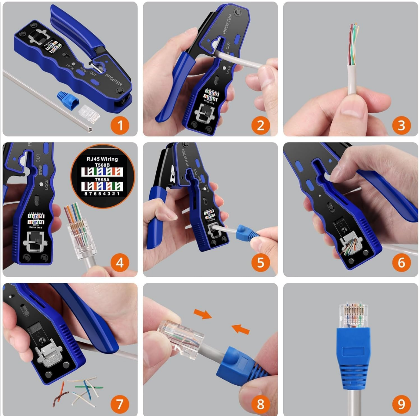
Image: A nine-panel sequence illustrating the complete process of preparing an Ethernet cable and crimping an RJ45 pass-through connector, from stripping to final connection.
