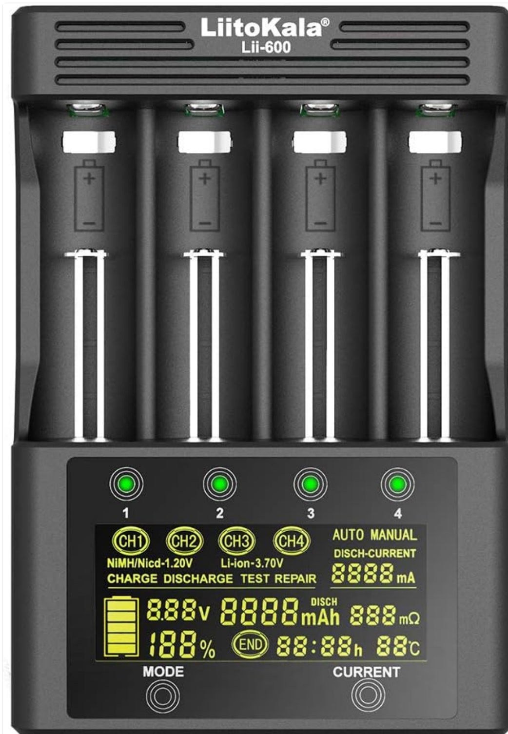
Image: The LCD display of the LiitoKala Lii-600 charger, providing detailed information on each battery slot, including current mode, voltage, capacity, internal resistance, and temperature.
