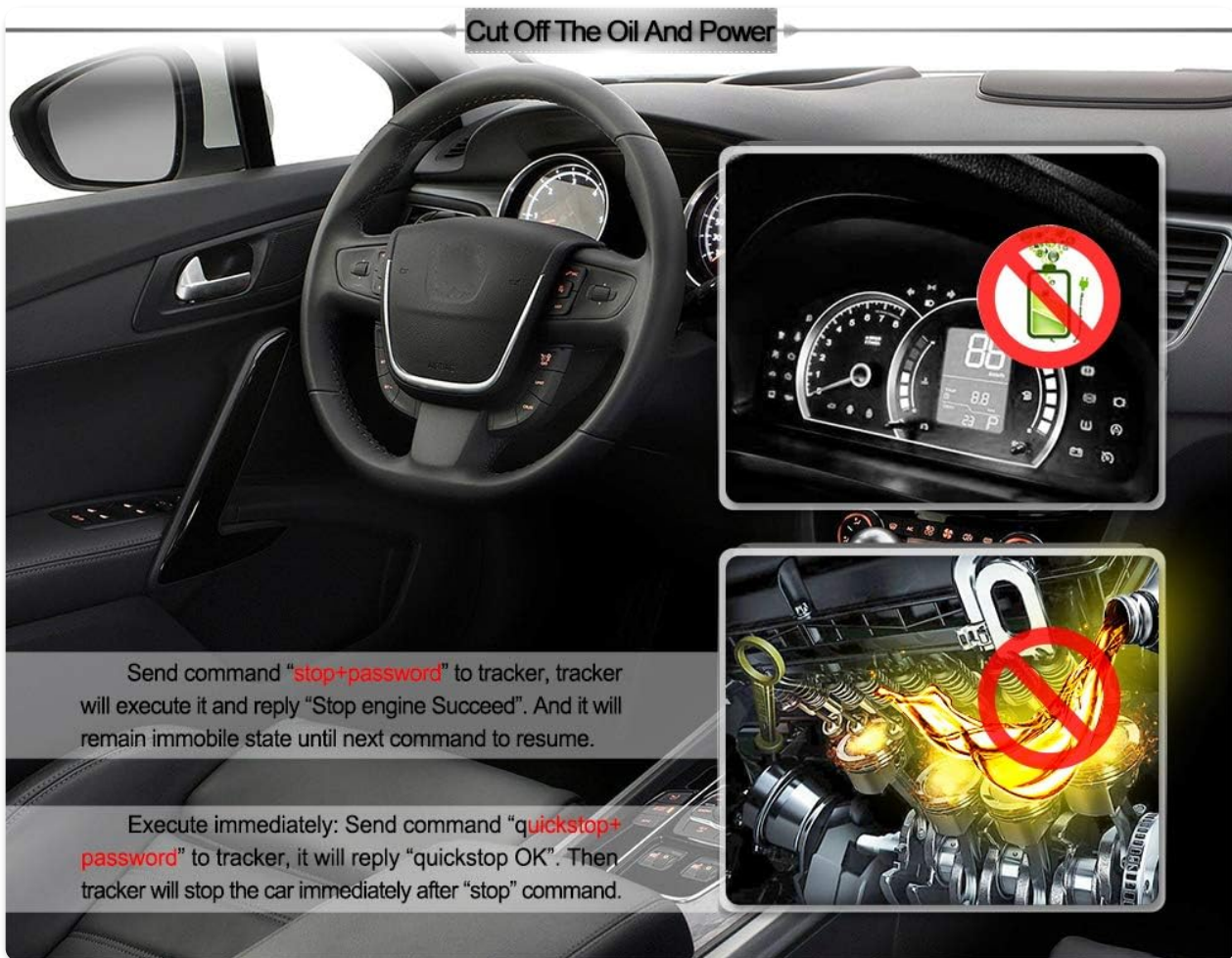
Image: A visual representation of the remote engine cut-off function via SMS command.
