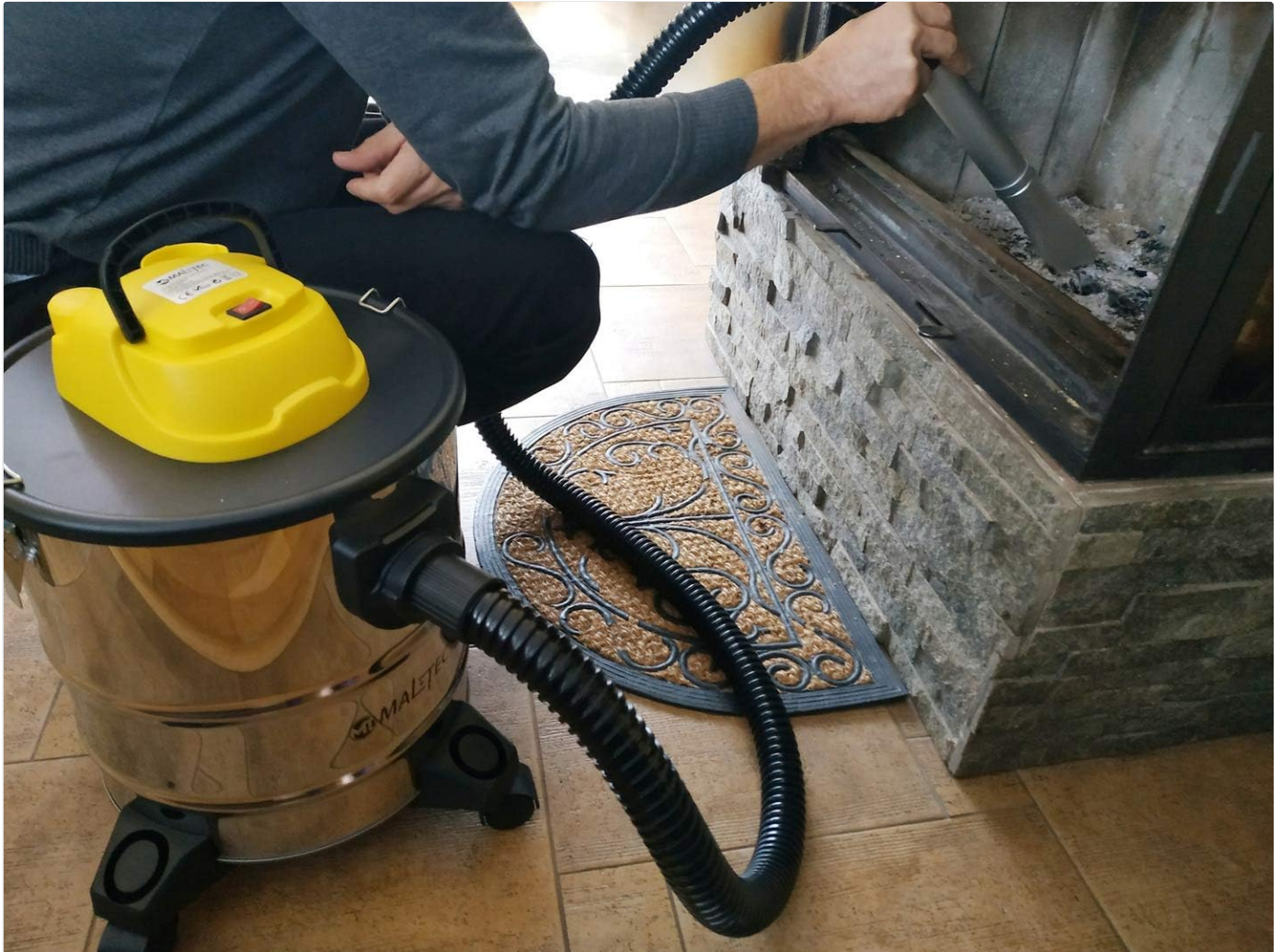
Image 6.1: Using the ash vacuum cleaner to clean a fireplace.
