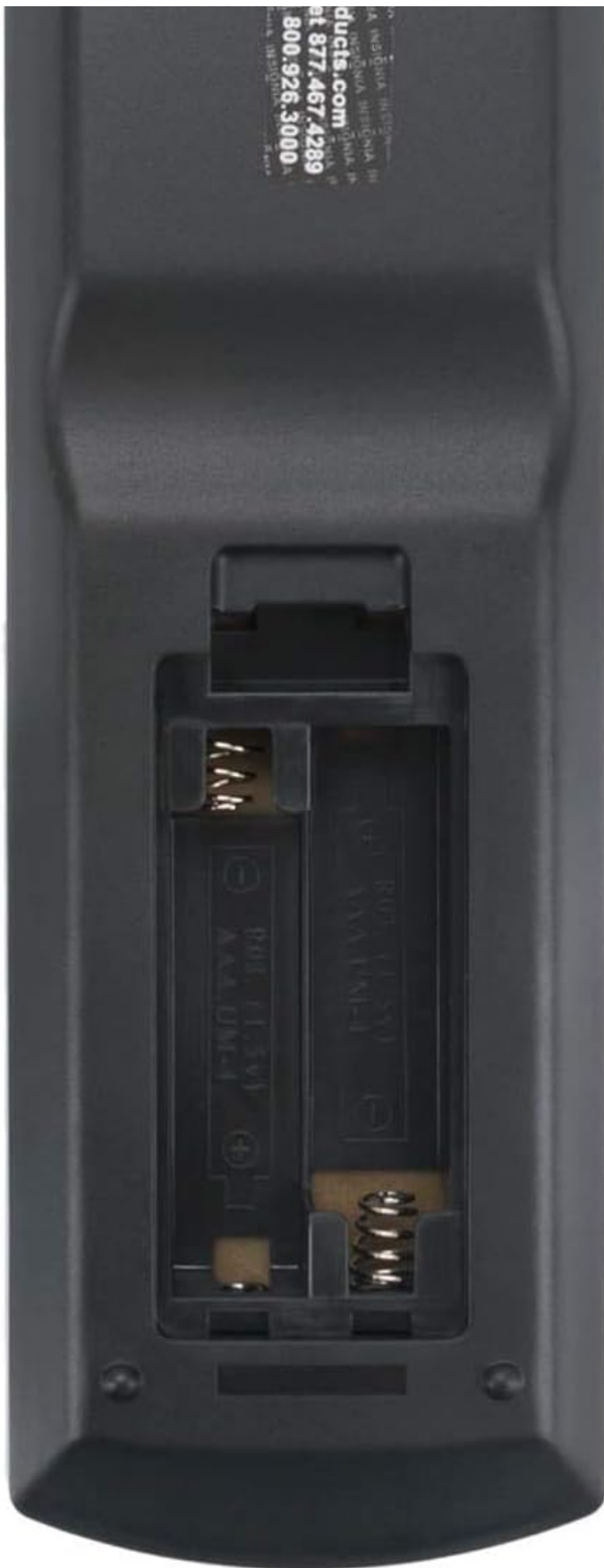
Image: Rear view of the ezControl Universal Remote Control with the battery cover removed, showing the battery compartment for two AAA batteries. This image illustrates the correct orientation for battery insertion.
