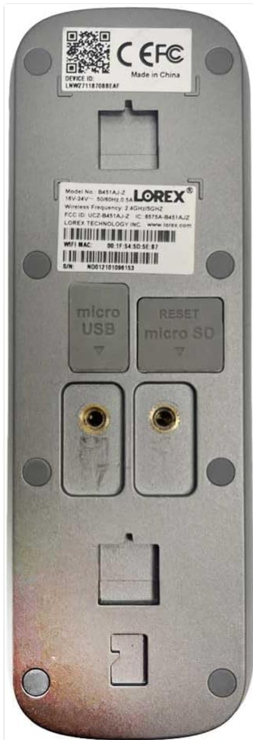
Image: Back view of the Lorex 2K Wired WiFi Smart Video Doorbell Camera. This image displays the Micro USB port, MicroSD card slot, Reset button, and power ports for wiring.
