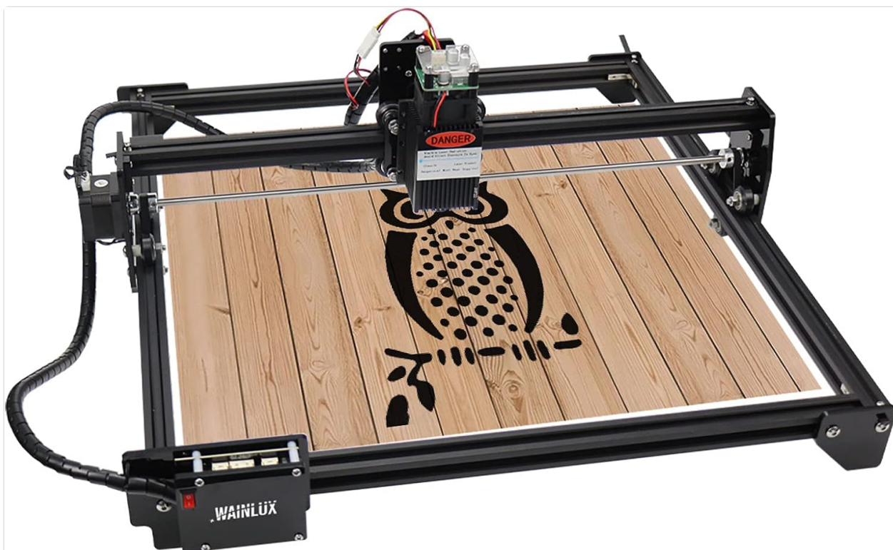
Figure 1: WAINLUX JL3 Laser Engraver in operation, demonstrating an engraved owl design on a wooden surface.
