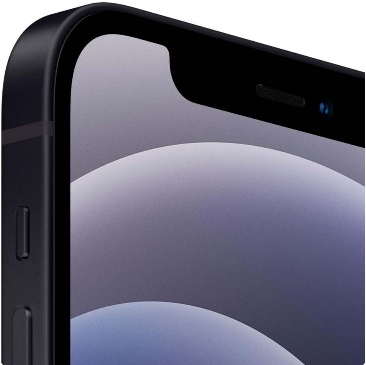
Figure 2: Close-up of the iPhone 12's display notch, housing the Face ID sensors and front camera.
