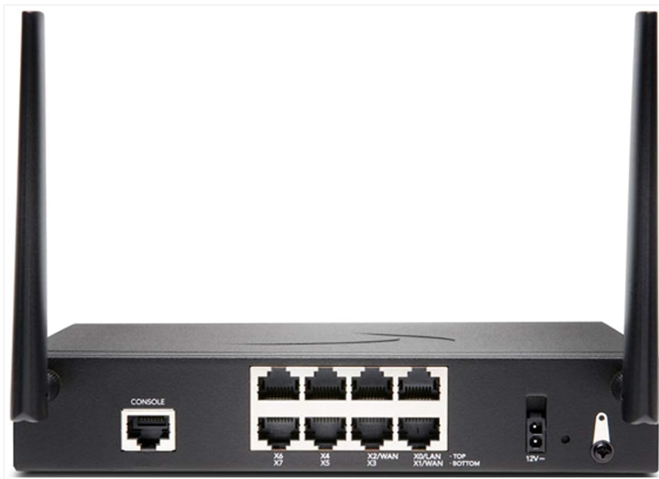
Figure 2.3.1: Sonicwall TZ370W Rear Panel. This image shows the rear view of the Sonicwall TZ370W, displaying the various Ethernet ports, console port, power input, and antennas.
