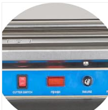
Image 3.3: Detailed view of the control panel, featuring the cutter switch, power indicator, and temperature adjustment knob.
