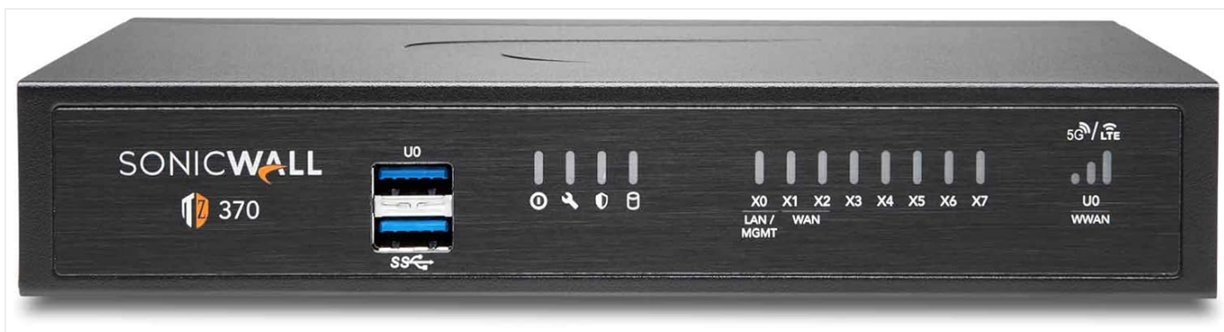
Figure 2.0: Front view of the SonicWall TZ370 Network Security Appliance, showcasing its compact design and front panel indicators.
