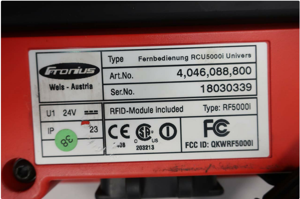
Figure 4: A detailed close-up of the product label located on the RCU 5000i. This label displays critical information such as the model type ("Fernbedienung RCU5000i Univers"), Article Number (Art.No. 4,046,088,800), Serial Number (Ser.No. 18030339), power requirements (U1 24V), IP rating (IP23), and compliance markings (CE, CSA, FC). It also indicates the inclusion of an RFID-Module, Type: RF5000i.
