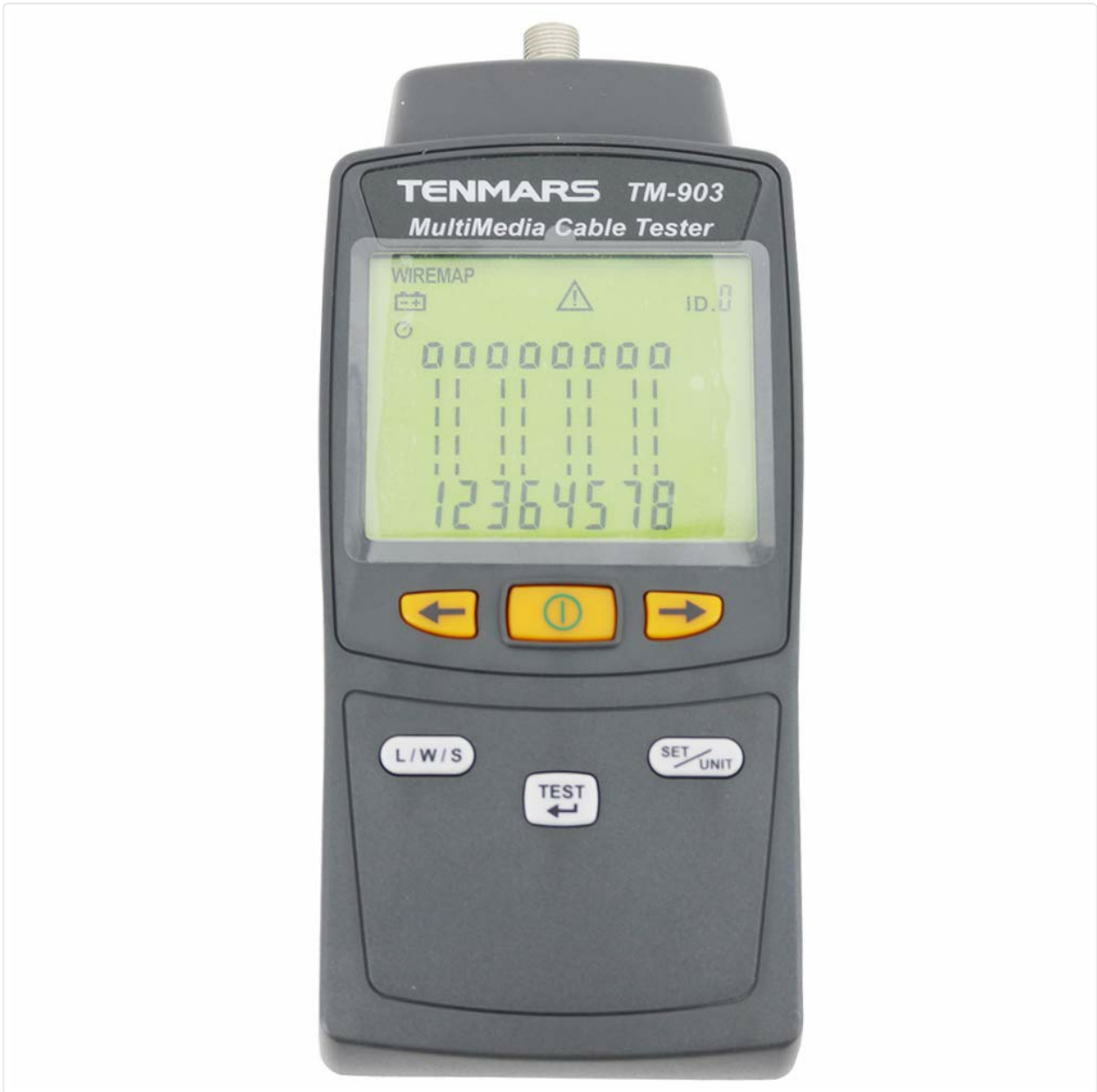
Figure 1: Front view of the TM-903 tester. The LCD displays test results, and the yellow buttons below control navigation and power. The 'L/W/S' button selects test modes, and 'SET/UNIT' adjusts settings or units.
