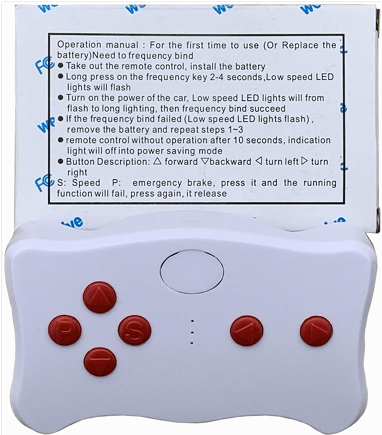
Figure 4.1: The reverse side of the weelye remote control, displaying the frequency matching procedure and button descriptions.
