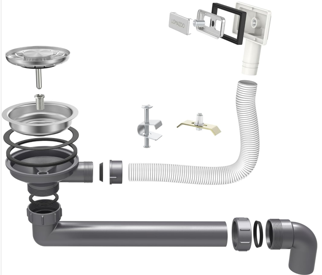
Figure 3.1: Exploded diagram showing all components included for the LOMAZOO sink installation, including the sink, drain assembly, and mounting hardware.
