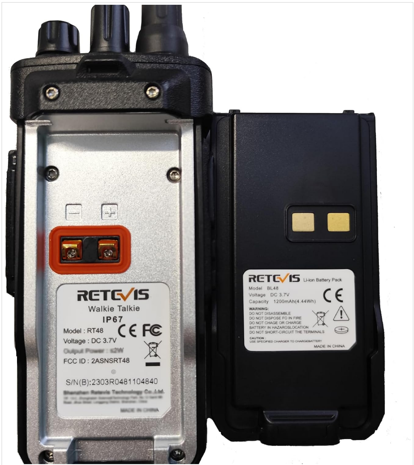
Figure 4: Rear view of the RT48 showing battery compartment.
