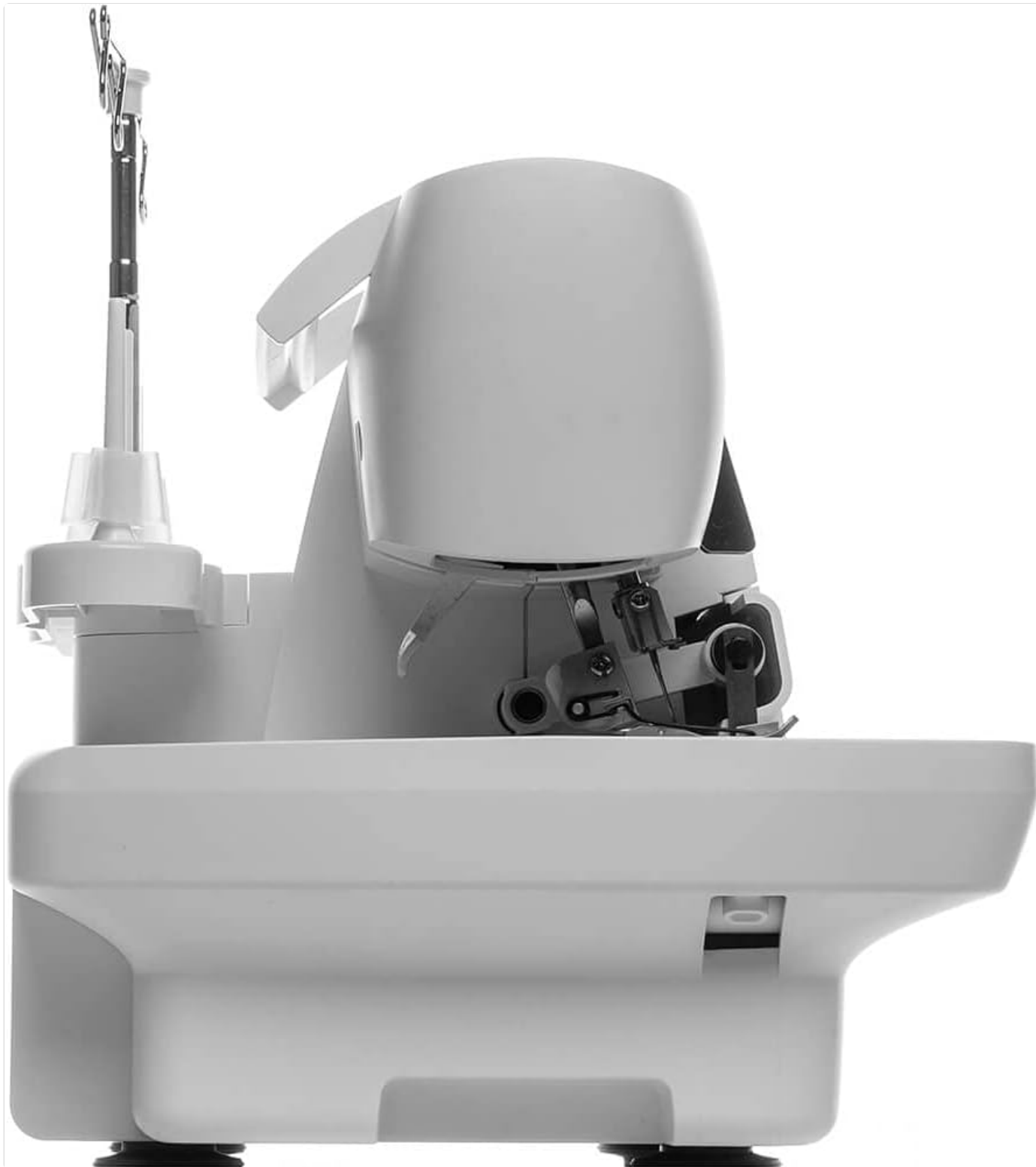
Figure 4.1: The SINGER S0100 with its free arm exposed for sewing cylindrical items.
