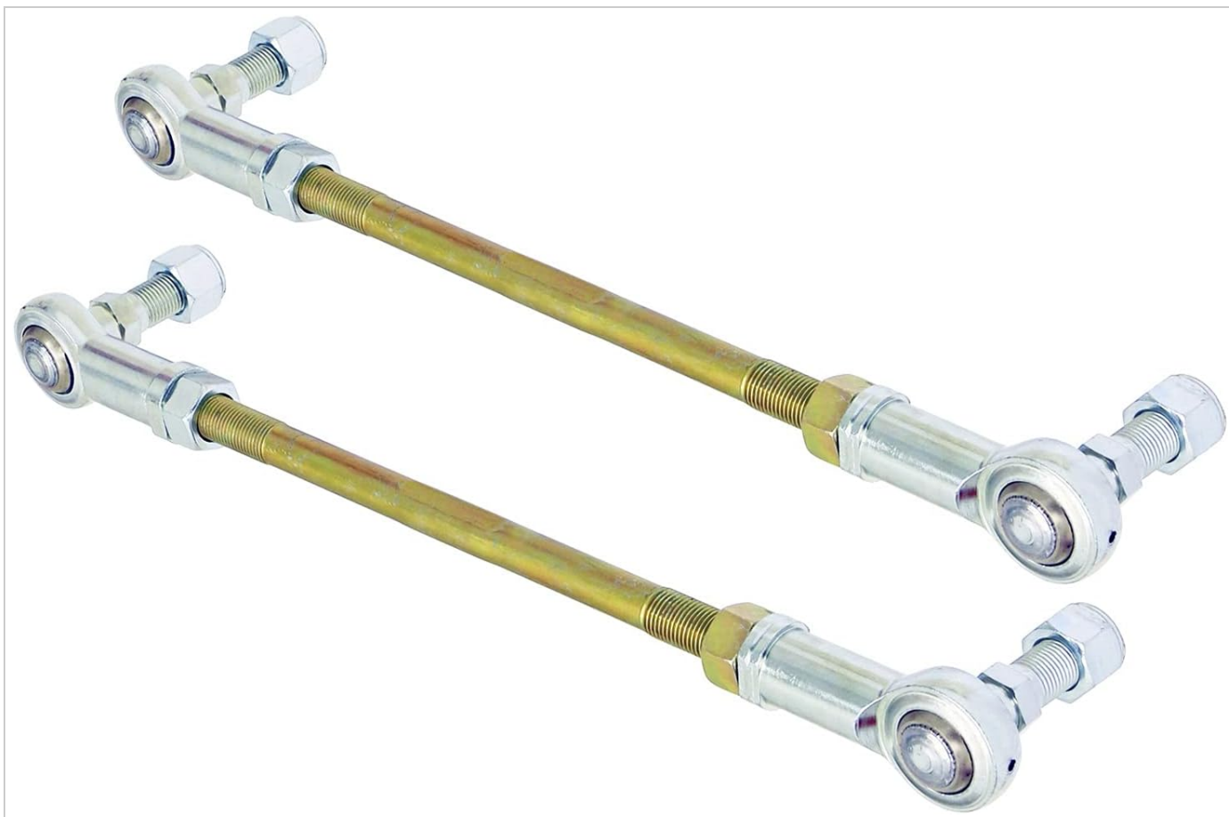
Figure 1: Rock Jock CE-99002 AntirockEnd Link Kit components. This image displays the two AntirockEnd Link assemblies included in the kit. Each assembly consists of a threaded rod, a spherical bearing at each end, and securing nuts. These components are designed for connecting the sway bar to the vehicle's suspension.
