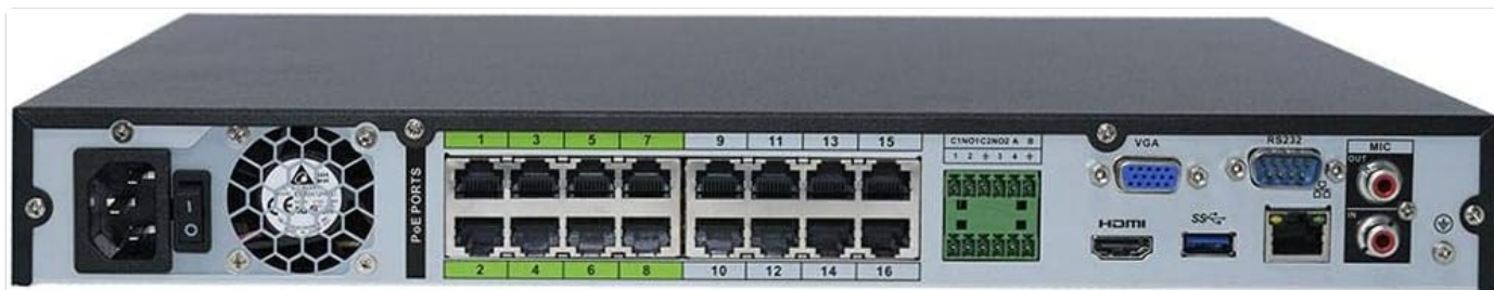
Figure 3.2: Rear panel of the Montavue 16-Channel NVR. This image displays the various ports including PoE ports, HDMI, VGA, USB, and audio inputs/outputs.
