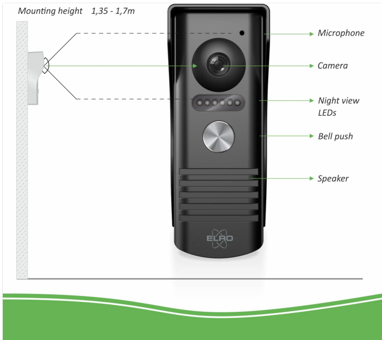
Figure 3: Doorbell unit components and recommended mounting height.
