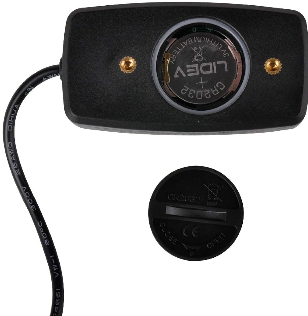
Image 4.1: Detailed view of the battery compartment and the CR2032 battery for replacement.
