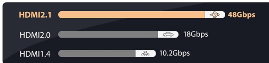
Image: Diagram illustrating the 48Gbps high-speed transmission capability of the HDMI 2.1 switch compared to older HDMI versions, emphasizing smooth performance for 8K content.
