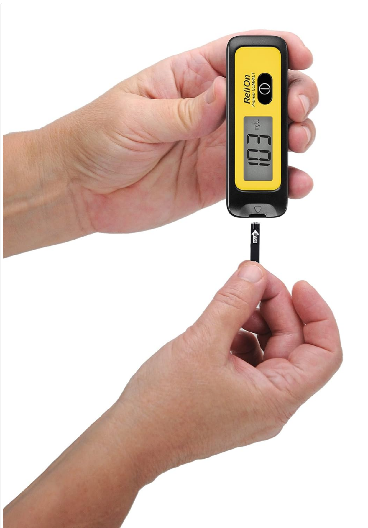
Image 4.1: Proper technique for inserting a test strip and preparing to apply a blood sample. The image shows a hand holding the ReliOn Premier Compact meter with a test strip inserted, while the other hand prepares a fingertip for lancing.
