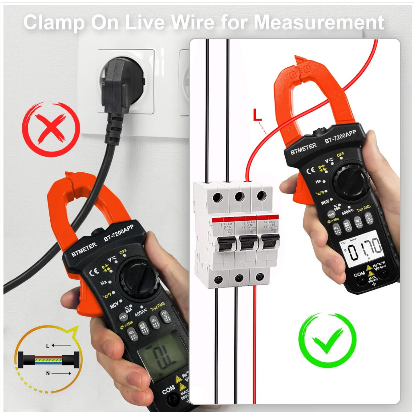
Figure 2: Correct Clamping for Current Measurement. The image illustrates the importance of clamping around a single live wire, not both live and neutral, to obtain an accurate current reading. An AC splitter can be used to separate conductors.
