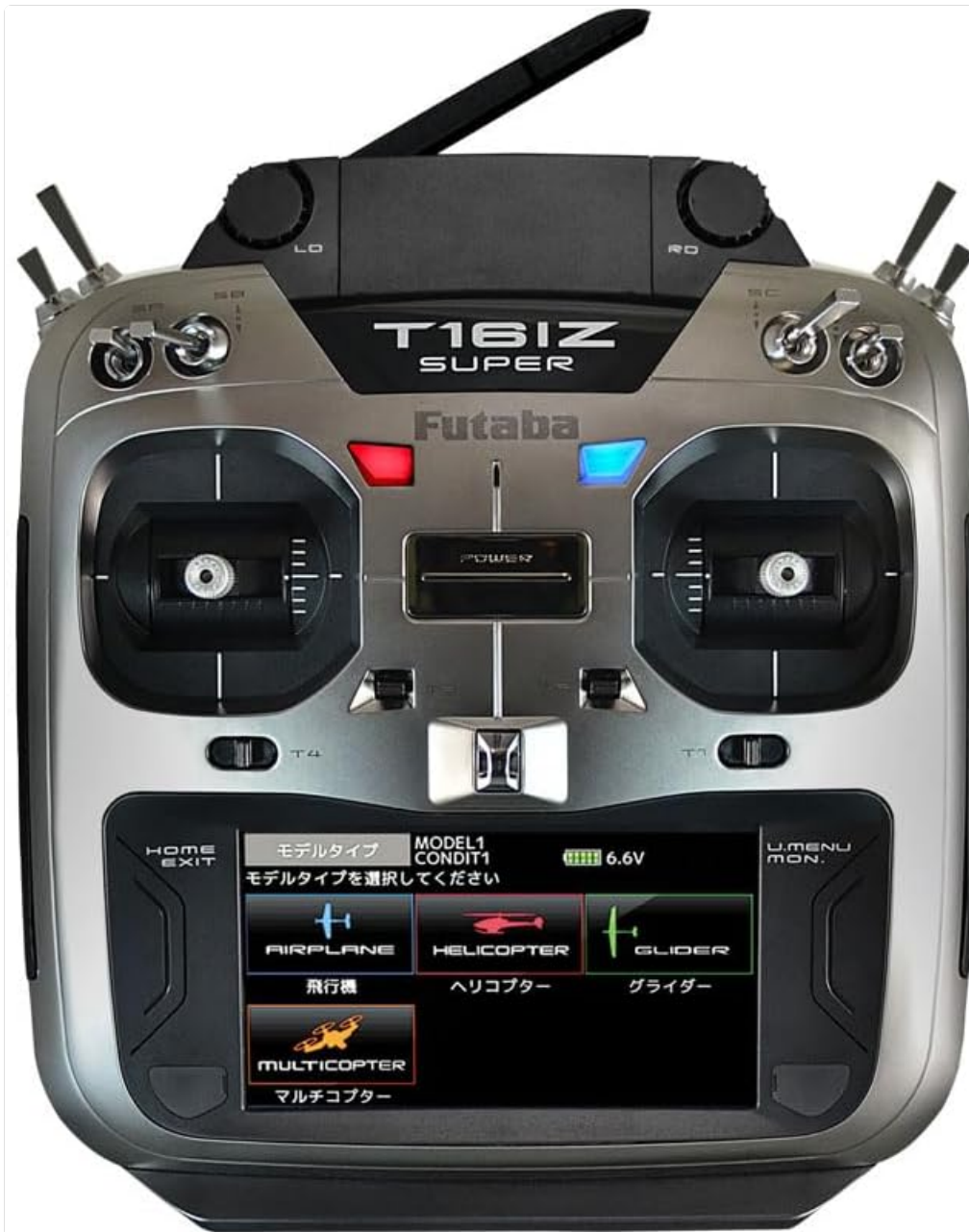
Figure 2: The FUTABA 16IZ Super Transmitter. This image highlights the transmitter's ergonomic design, dual spring-loaded sticks, and the integrated color display, which shows various settings and telemetry data.
