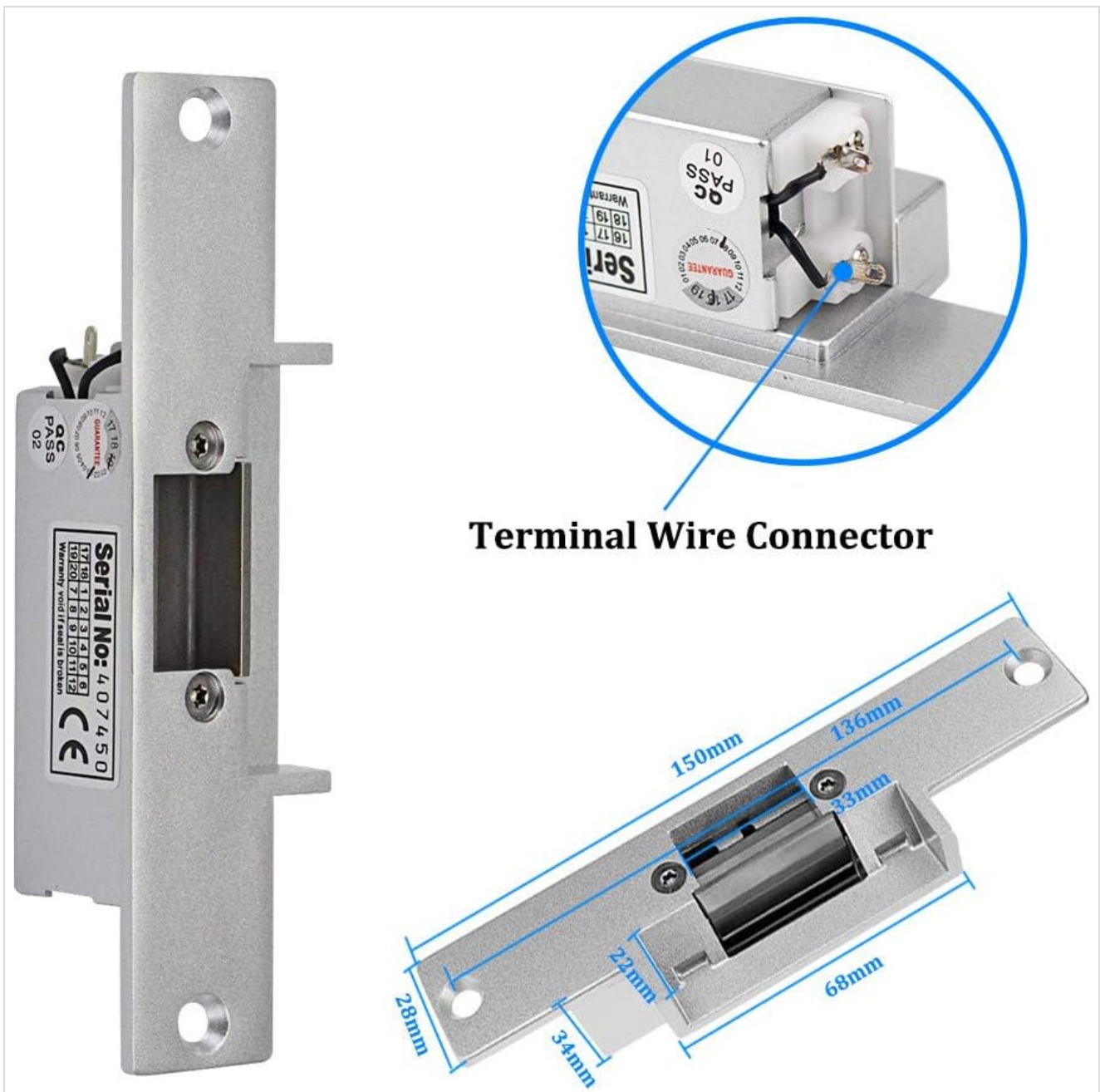
Image 2.3: Detailed view of the electric strike lock, including its dimensions and terminal wire connector.
