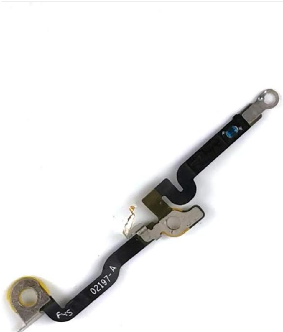
Image: A top-down view of the MEEFIX Bluetooth Antenna Flex Cable, showcasing its design and connectors.
