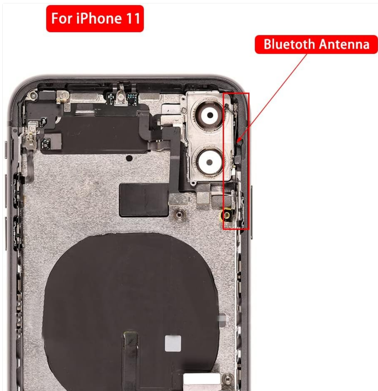
Image: The MEEFIX Bluetooth Antenna Flex Cable shown installed within the chassis of an iPhone 11, highlighting its typical location near the top right corner.
