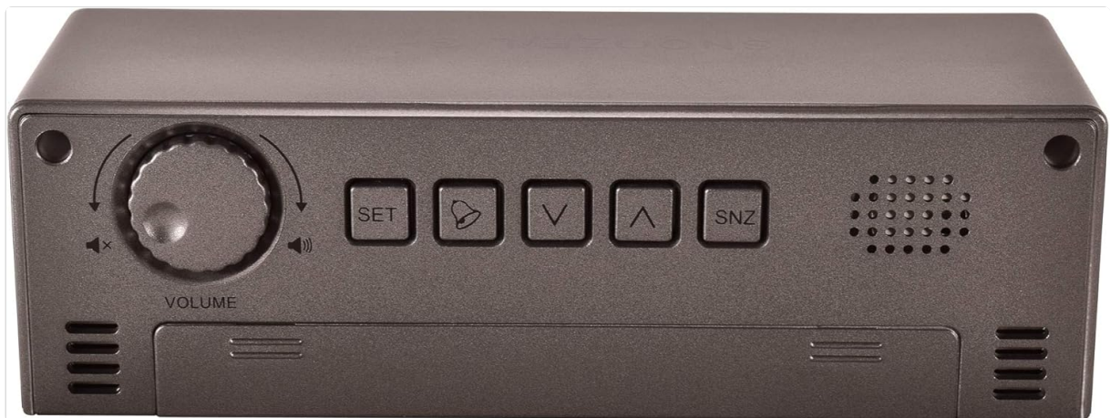
Figure 3: Rear view of the Acctim Karminski Digital Alarm Clock, highlighting the control buttons and volume knob.
