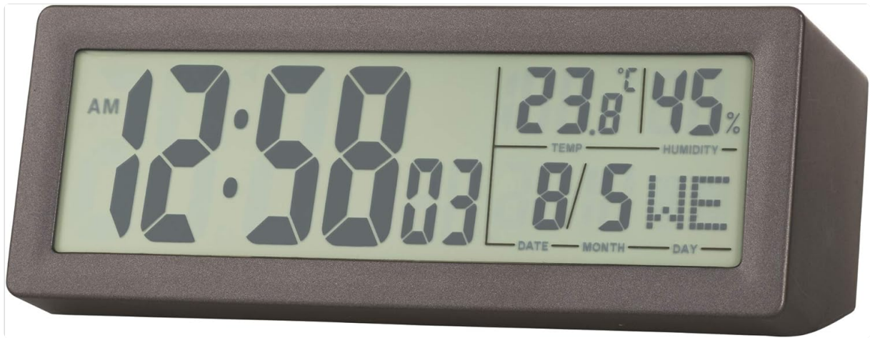
Figure 1: Front view of the Acctim Karminski Digital Alarm Clock displaying time, date, temperature, and humidity.
