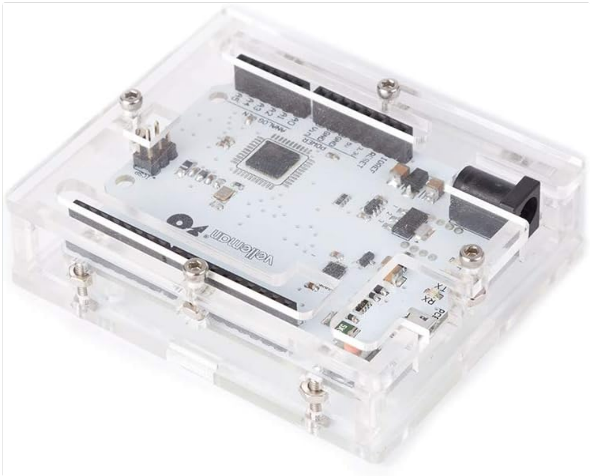
Image 1: Arduino UNO R3 board positioned on the bottom acrylic panel.
