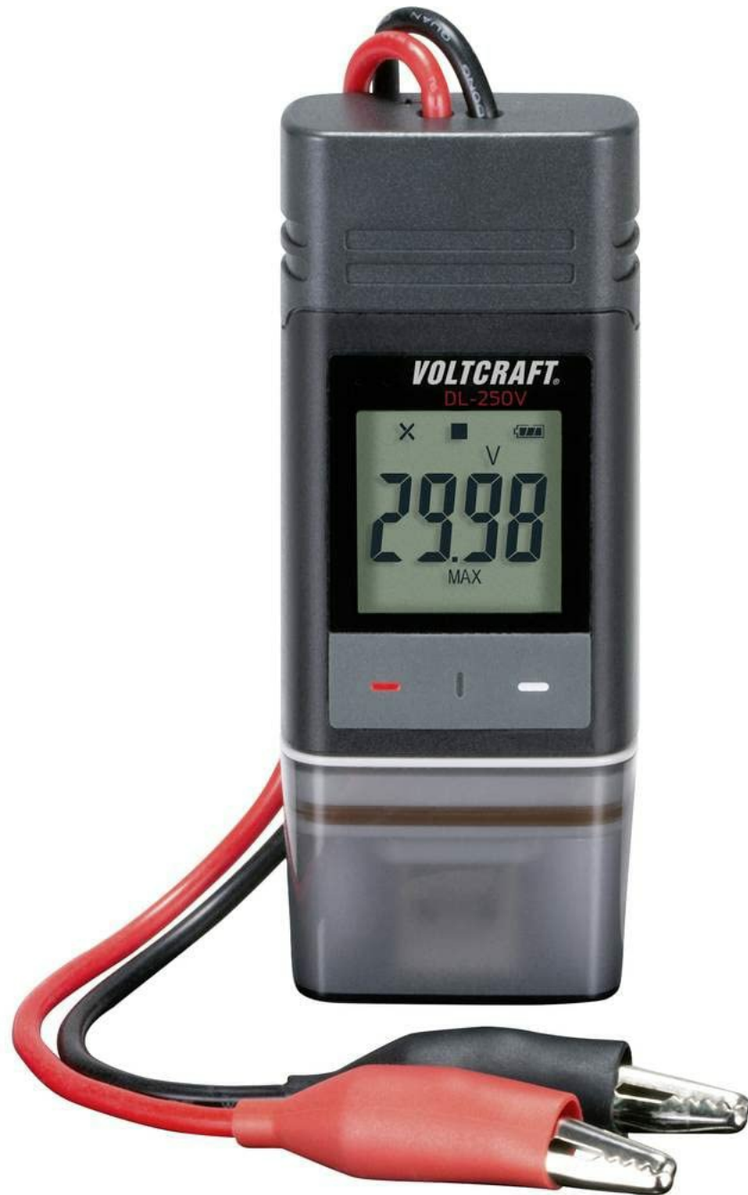
Figure 2: Upright view of the DL-250V, highlighting the LCD screen and the input terminals for the voltage probes.
