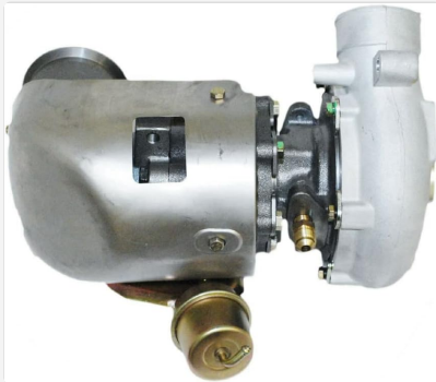
Figure 4.2: Side view of the turbocharger, highlighting the wastegate actuator mechanism. The actuator controls exhaust gas flow to regulate boost pressure.
