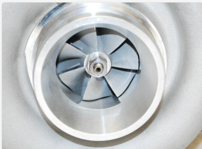
Figure 4.7: Detailed view of the compressor wheel, responsible for drawing in and compressing air before sending it to the engine's intake manifold.
