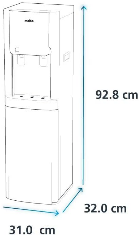
Figure 3: Diagram illustrating the dimensions of the Mabe EMDPCCB1 Water Cooler.
